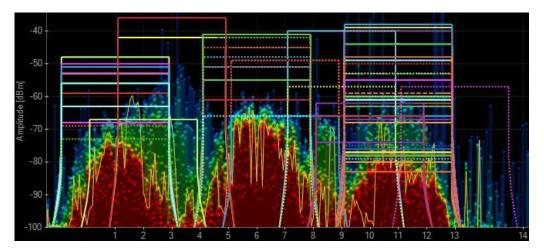
The figure above shows a completely saturated 2.4 GHz band, used by 802.11b/g/n, Bluetooth, wireless telephones, baby monitors, security cameras, etc. It is also affected by microwave ovens. Notice the amount of energy (in red) that is spread across the entire radio frequency spectrum (the horizontal axis).
