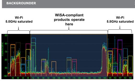
As can be seen in the above figure, the 5 GHz band is much less crowded. Using it requires dedicated 5 GHz equipment and Dynamic Frequency certification.
