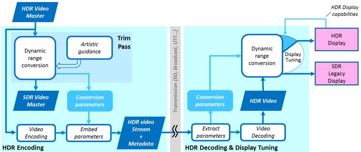
The process starts from an HDR video master. This HDR master must be graded on a high-dynamic-range display with high peak luminance and low black level. In the case of live production, such display should be used to monitor the HDR video master. The HDR video master is encoded. Typically, an HEVC video encoder will be used, with SMPTE ST 2084 as EOTF.
