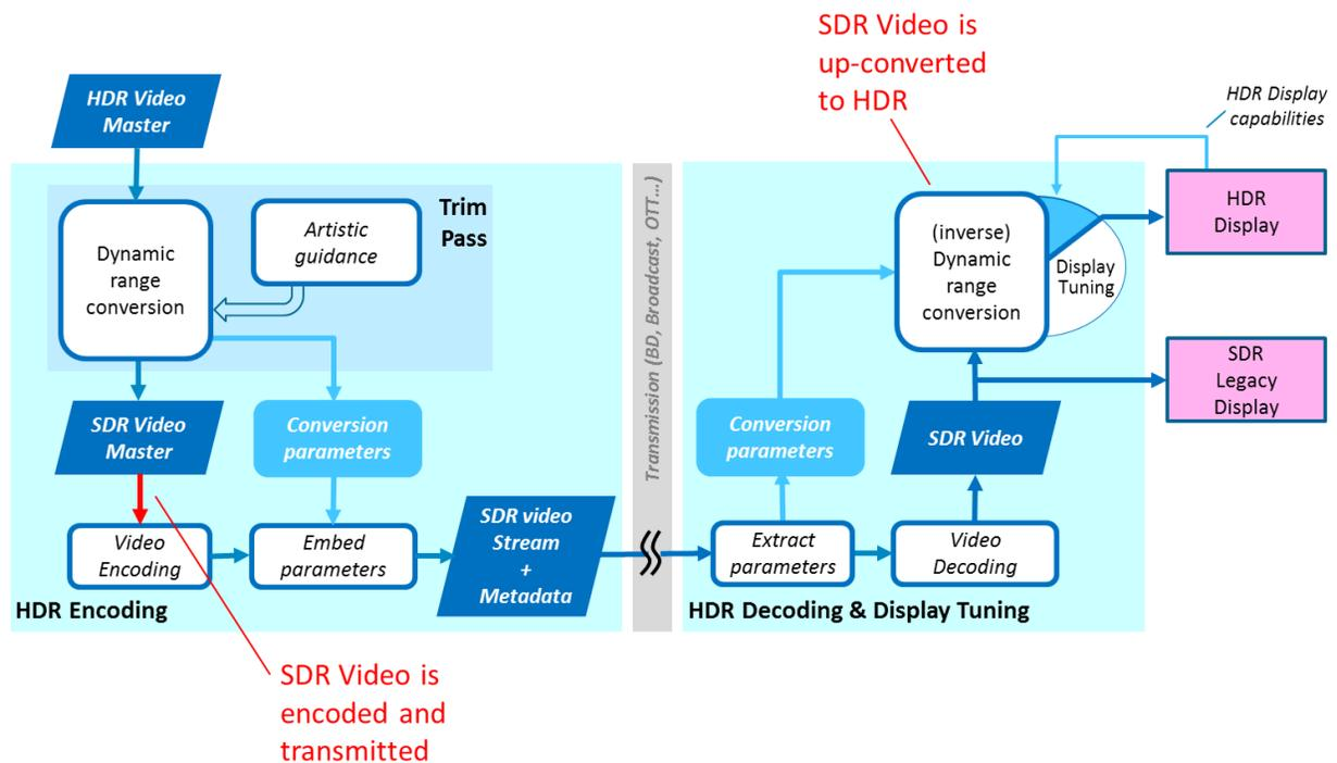
The decoder receives the SDR signal that can go directly to an SDR display. An 'HDR-aware' decoder retrieves the conversion parameters from the video stream. Now, the *inverse* dynamic range conversion has to be applied to the video to obtain the HDR video.
